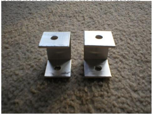
I made my brackets out of stock aluminium I bought at home depot. Drill one hole on the bottom to fit the factory fastner and the second hole on top to fit the bolt you are using to mount the bracket.
