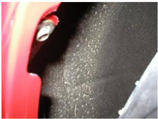
3. Remove the five black plastic fastners three across the top by the trunk and 2 on the bottom by the mufflers.
